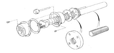
Single Tube Electric Immersion Heater
