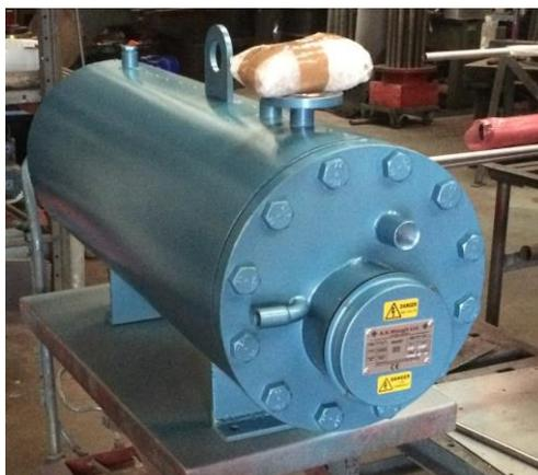
Watts Rating (on electrics) between 5 and 8 W/in<sup>2</sup> ( 0.77 and 1.22 W/cm<sup>2</sup>)
